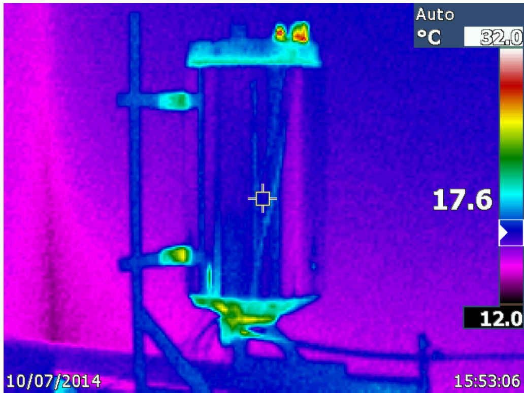
Figure 21: Thermal image for geyser B in vertical orientation – Side view.
