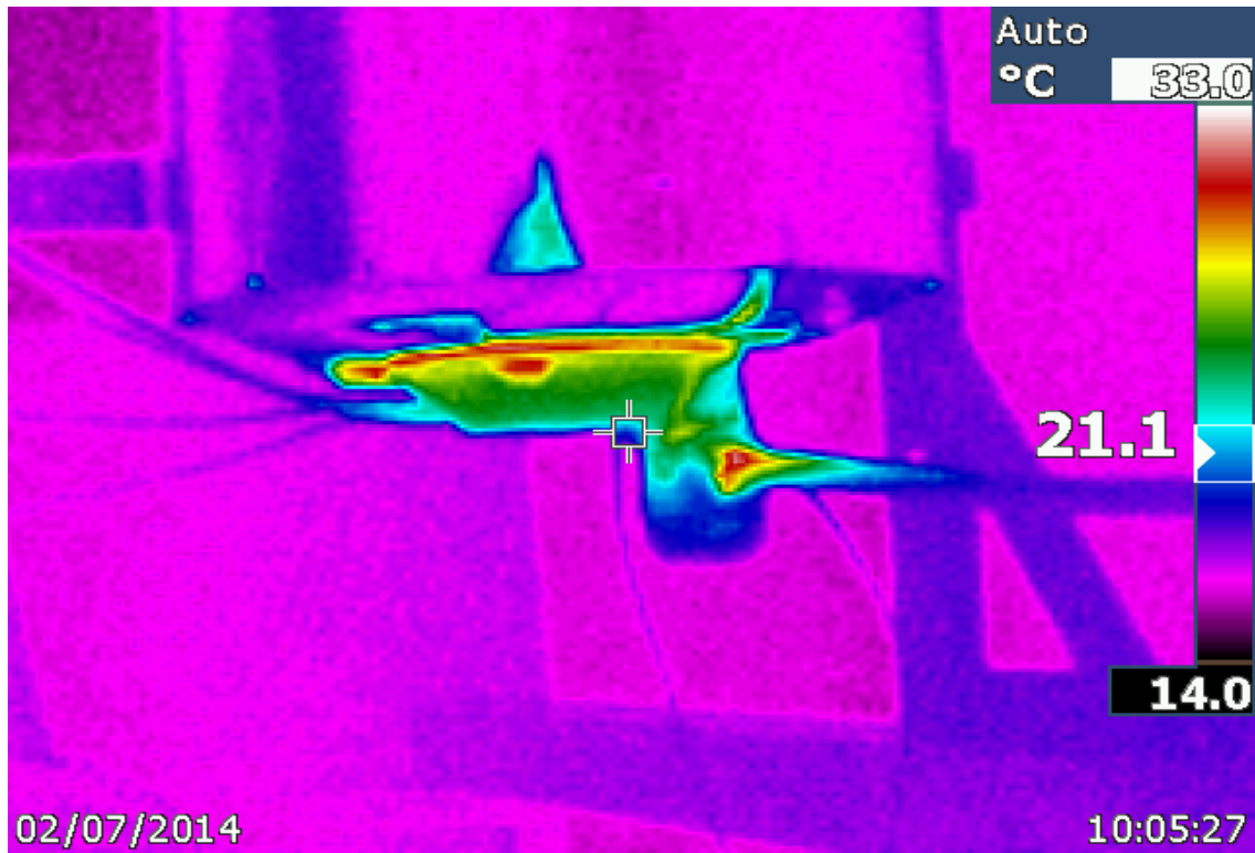
Figure 35: Thermal image of geyser C in vertical orientation – Inlet end.
