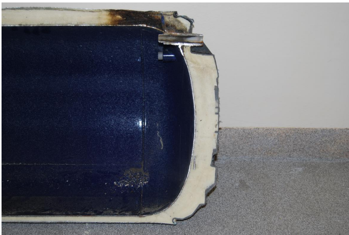
Figure 14: Cross section of geyser A – Outlet end. The burn marks are a result of the cutting process.
